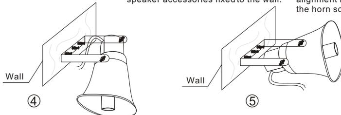
4. Figure, a 90-degree vertical installation fixed in the wall. Such as the need to change the security point of view can be moved loaded speakers.
