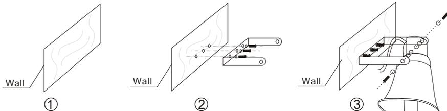
1. Speaker weight of 1.6Kg, must be chosen Solid body by force, to avoid unstable speakers falling or injuries.
