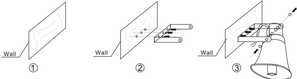
1. Speaker weight of 2.1Kg, must be chosen solid body by force, to avoid unstable speakers falling or injuries.
