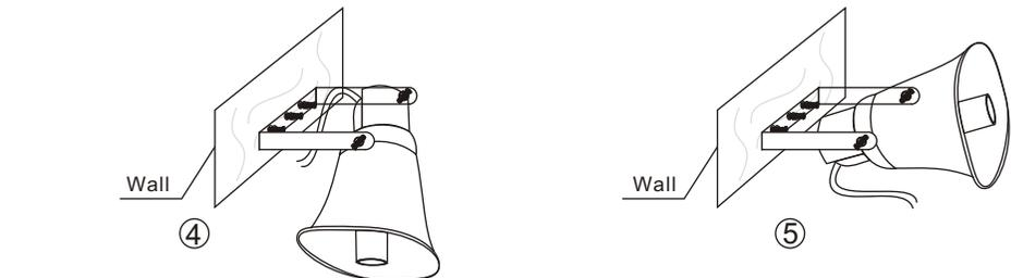
4. Figure, a 90-degree vertical installation fixed in the wall. Such as the need to change the security point of view can be moved loaded speakers.
