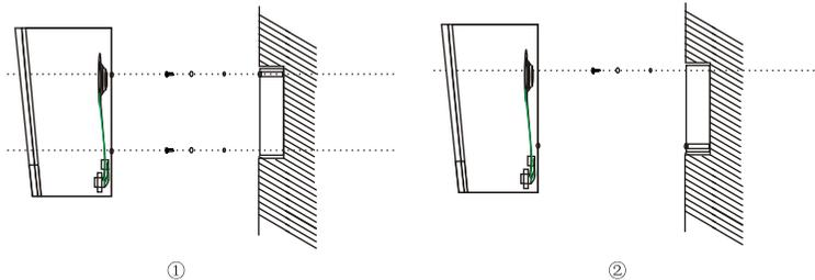
Step 1: Open a hole on the wall which is more larger than bottom box and install the bottom box on the wall, the distance between the orientation hole of the bottom box is 101mm, fix up the bolt and hang the speaker to the orientation hole.
